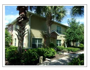
SIDE ELEVATION VIEW – The side entryway gables are not structurally connected to the main roofing system. They are attached to the reinforced walls.
